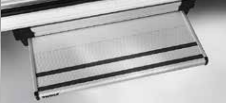
7 Entry step with electronic deployment function
