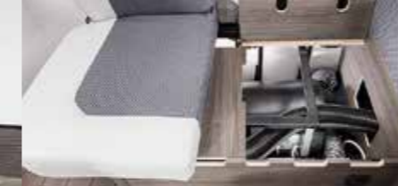
4 Diesel heating in the living area
