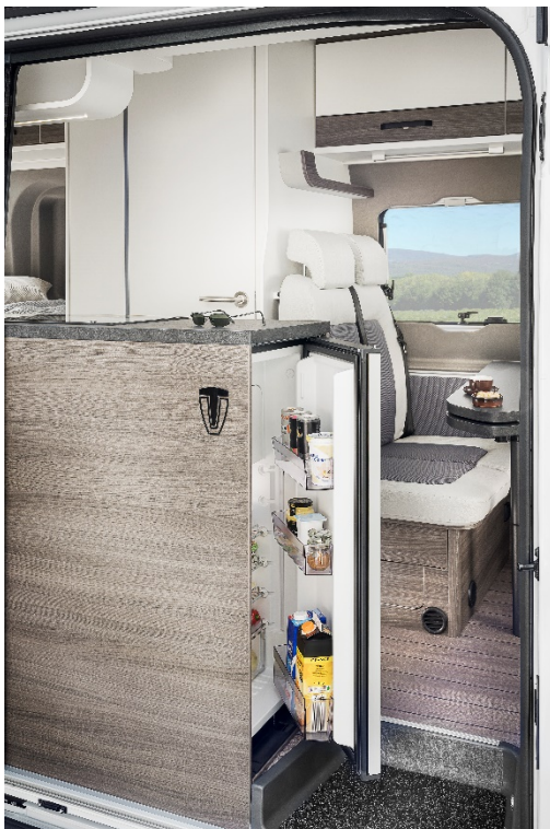
Caption: Thanks to the double hinge, the refrigerator door can be opened in both directions.
