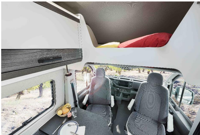
Caption: The GRP high roof extends the space available.
