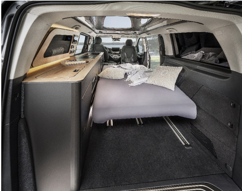
Caption: The bench seat can be converted into a sleeping area or even removed completely as required.
